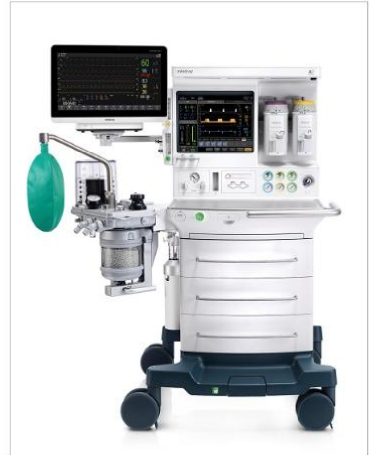
The Mindray A7, one of the products that received the software revision that resolved the low-minute-volume default issue. (Image courtesy of Mindray.)
